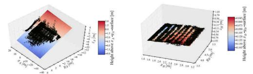
Figure 5: Left: Linear approximation of the ground surface to determine a scene's global orientation. One can observe the large variation in z coordinates creating the need for local regression surfaces for accurate height estimation. Right: Local regression surface along with the corresponding ground points from the point cloud for one plot. From Khanna et al. 2015.
