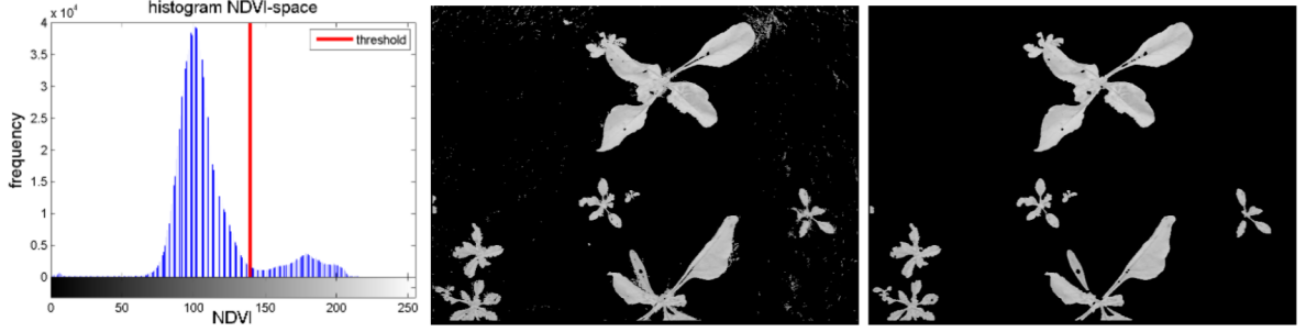
Figure 3: Left: Histogram of \mathcal{I}_{NDVI} and threshold (red) for separating vegetation. Middle: masked NDVI after threshold operation containing errors. Right: final vegetation mask after optimization.
