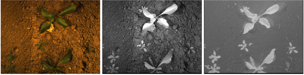
Figure 2: From left to right: Raw input RGB and NIR image and processed NDVI image.
