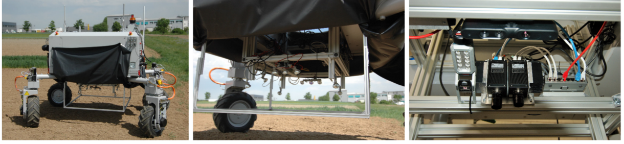
Figure 8: Left/Middle: BoniRob V3 with support structure for mounting the camera as well as the shading and attached halogen spots for illumination of the shaded space under BoniRob. Right: Two JAI AD-130 GE cameras mounted on support structure straight looking downwards.
